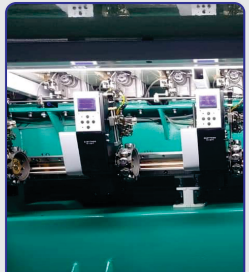
8 STATION AUTOMATIC BOBBIN CHANGER
